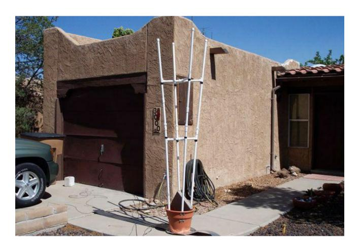
The above picture is the Flower pot antenna completely assembled bfore painting it with flat black paint. The flat black paint job makes it almost disappear in a patio enviorment but other colors could be used to make it match up with it's background. It is a excellent way to hide atennas in plain site.
