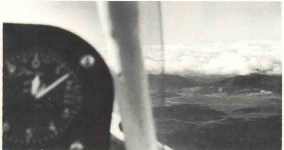
The Evans VP-1 over the Laguna Mountains at an altitude of 10,140 ft., about the service ceiling for the airplane operating with a 1500-cc. engine at a gross weight of 725 lbs.
