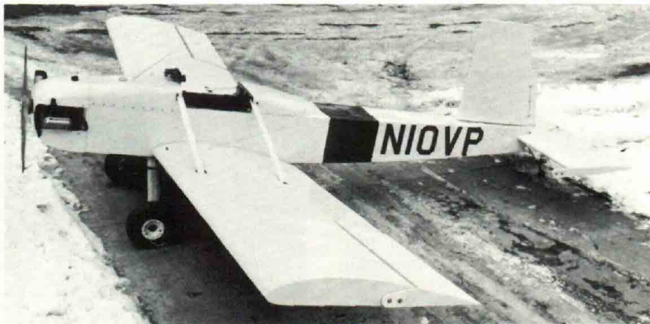
Flown for the first time in February was this Volksplane, N-10VP, built by G. Michael Even (EAA 52512) of 912 Shorewood Court, Lake of the Woods Estates, Dunlap, Ill. The engine is a 40 hp conversion out of a 1964 Volkswagen. The craft is painted Daytona white and has a black German cross over a red fuselage band. While it appears to follow the plans in every respect, it does not have the turnover bar around the windshield.
