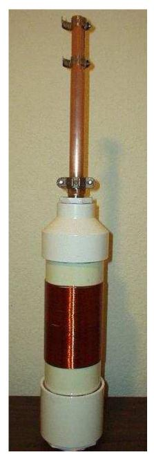
When mounting the completed antenna onto the mast, it should be obvious that the 1 ½" steel mast screws into the bottom of the coil form.
