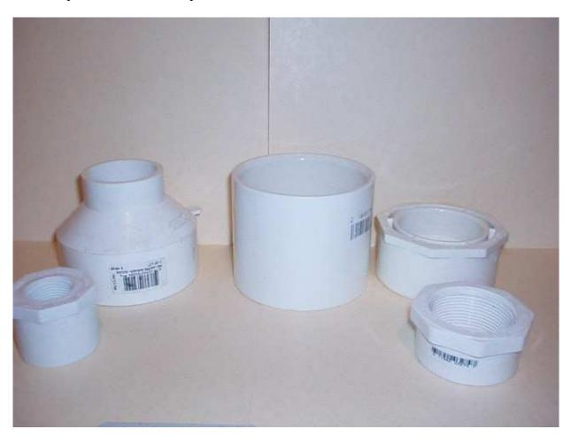
The first two parts will replace the original top cap on the coil form. The last three parts will replace the bottom cap on the coil form. Assembled, they will look like this picture.
