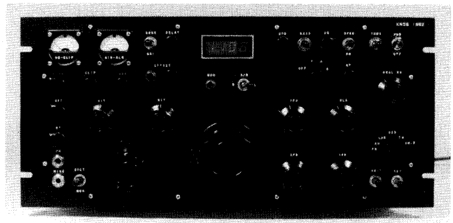
Fig 1—In my home-brew transceiver shown here, the AGC switch is labeled OFF-F-M-S. The SQUELCH (down) switch is part of the OPERATE (up) and STANDBY (center) switch, which is labeled merely OPER-SQ. The meters read signal level in dB and squelch integrator charge. Not shown here are the three separate transceiver front-end sections for MF/HF, 6 meters, and 2 meters.
