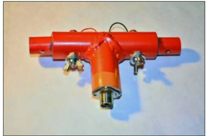
Finished center-fed "Tee," assembled, with SO-239 connector for RG-58 50Ω coaxial feed line input.
