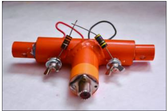
Feed "Tee" and balun with 330+470Ω resistors to simulate 800Ω load of terminator for bench testing. Balun SWR 1:1 @ 3.5MHz to 1.2:1 at 30 MHz.
