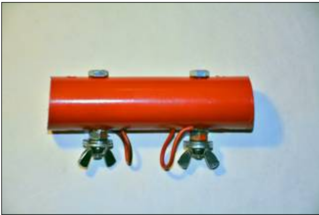
Terminator resistor unit, assembled. Internal resistors (800Ω at 10W) inside 3/4" O.D. x 5" PVC tubing; 1/4-20 bolts and wingnuts for dipole connections.
