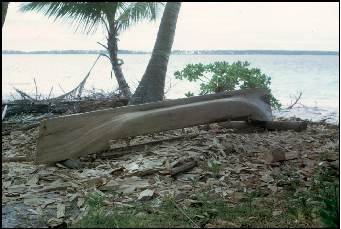
The Outrigger for our Sail Boat being built by the Island Carpenter
