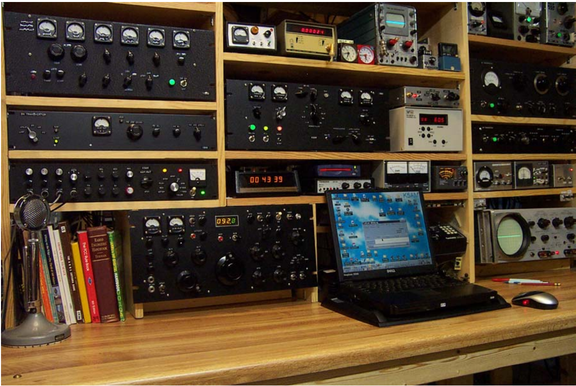
Photo 24A. K5AM homebrew station. The Hapirat is above and to the left of the homebrew transceiver. Above the Hapirat is a transverter and a 200 watt tetrode amplifier for 144 MHz. Above the 6-digit clock is the HF section of the transceiver. Above the old HP scope, on rack panels, are two 50 MHz transverters, vintage 1963 and 1989. In the upper right corner is a small 50 MHz amplifier built while in high-school in 1951, still in constant use today. To the right is the 6 foot rack with kW amplifiers for 6 meters, HF, and 2 meters, vintage 1961, 1971, and 1995.
