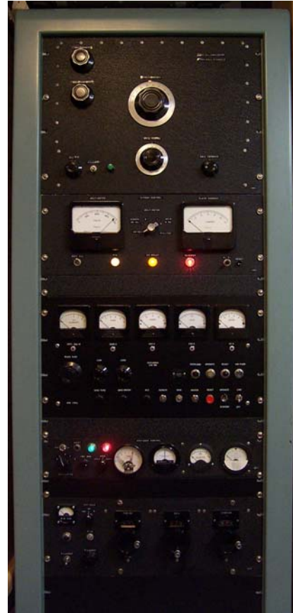
Photo 24A. K5AM homebrew station. The Hapirat is above and to the left of the homebrew transceiver. Above the Hapirat is a transverter and a 200 watt tetrode amplifier for 144 MHz. Above the 6-digit clock is the HF section of the transceiver. Above the old HP scope, on rack panels, are two 50 MHz transverters, vintage 1963 and 1989. In the upper right corner is a small 50 MHz amplifier built while in high-school in 1951, still in constant use today. To the right is the 6 foot rack with kW amplifiers for 6 meters, HF, and 2 meters, vintage 1961, 1971, and 1995.
